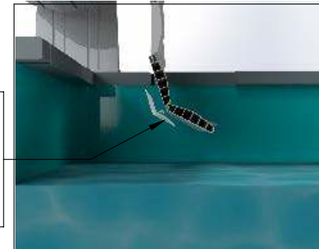
Blade guide ski: Slide the PVC ski for clipping in the female part giving the inclination of the first blade at \approx 45^\circ
